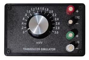
Totalcomp Transducer simulator (TS-16) are used to test digital weight indicators in weighing equipment. The indicator can be precalibrated prior to installing the load cells and using test weights to calibrate the scale. A indicator with set points can be tested to determine the accuracy.
